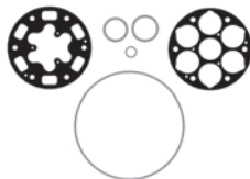
Includes: Cylinder Gasket (1), Head Gasket (1), Lip Seal O-Ring (1), Case O-Ring (1), Oil Drain Plug O-Ring (1), Control Valve O-Ring (1).
